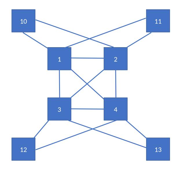
Many enterprise networks are organized with a set of backbone devices interconnected by using a full mesh of links.
