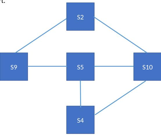
What is the spanning tree that will be computed by 802.1d in this network assuming that all links have a unit cost? Indicate the state of each port.
