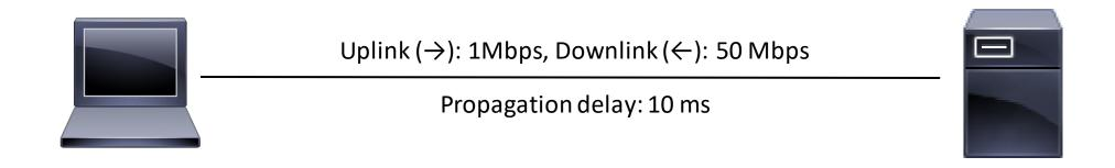
Duration of the retransmission timer in the alternating bit protocol?
