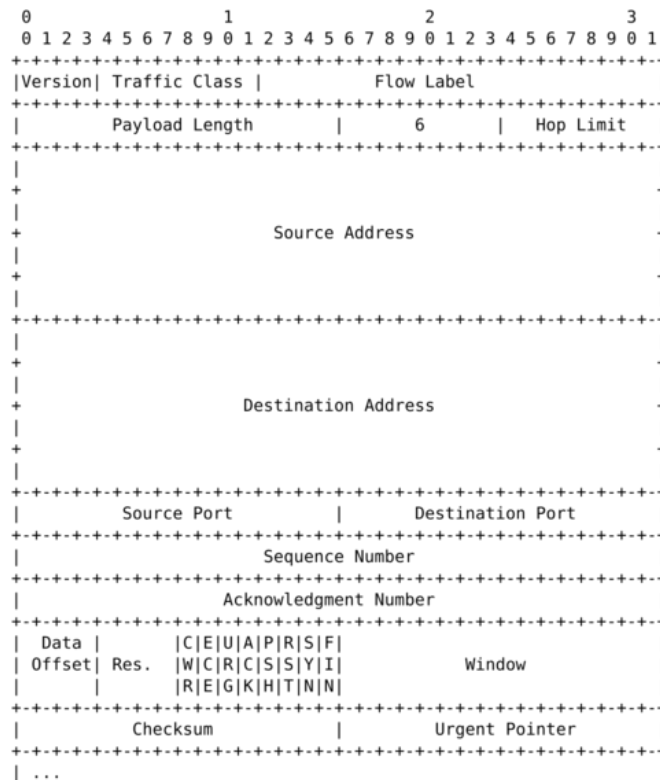
Fig. 45: An IPv6 packet containing a TCP segment
