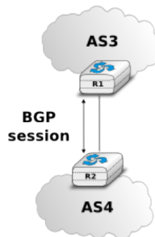
Fig. 70: A BGP peering session between two directly connected routers
