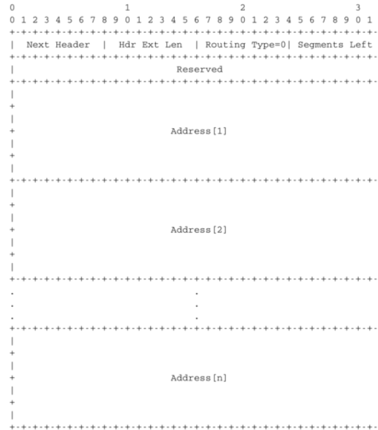
Fig. 50: The Type 0 routing header ( RFC 2460 )
