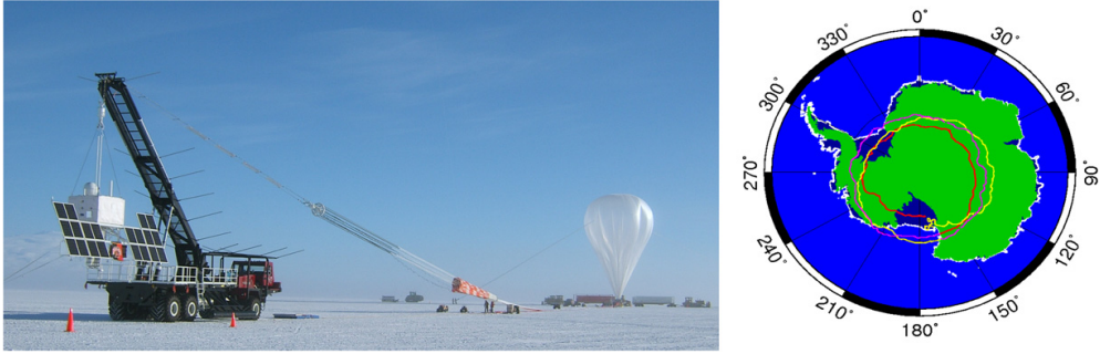
Fig. 16.4 Flight of the balloon experiment CREAM in Antarctica (from [887], with kind permission of Elsevier). Left: Launching the balloon the apparatus is moved on a vehicle following the floating balloon until the apparatus lifts off. Right: A flight track on which the CREAM apparatus has circled the South Pole three times in 37 days.
