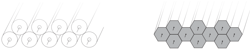
Fig. 7.35 Cross sections of round ( straw ) and hexagonal ( honeycomb ) drift tubes.
