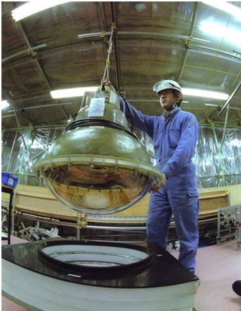
Fig. 10.12 Large photomultiplier tube (Hamamatsu R3600) with a cathode diameter of 51 cm for the Super-Kamiokande experiment. With kind permission of Hamamatsu Inc.
