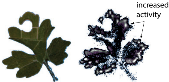
Fig. 8.71 Radioactivity distribution of a leaf marked with tritium, recorded by a DEPFET pixel detector [953]. (a) Photograph of the leaf, (b) grey-coded activity (lighter color represents higher activity).
