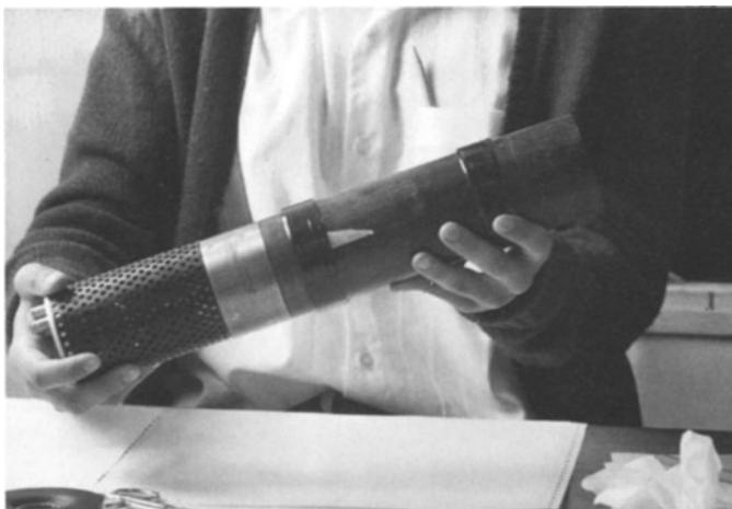
Fig. 9.14. Assembled scintillation detector
