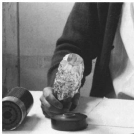
Fig. 9.12. Wrap scintillator loosely in aluminium foil
