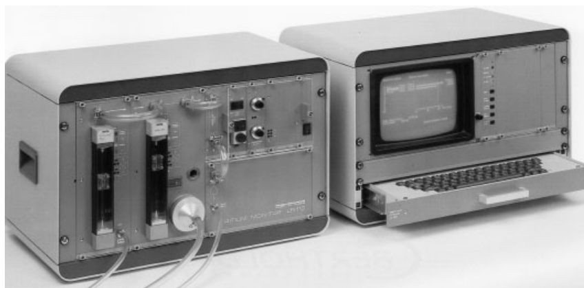
Fig. 10.9 Gas-flow proportional counter for monitoring tritium activity concentration in air. See text. (Courtesy Berthold Technologies USA, LLC.)
