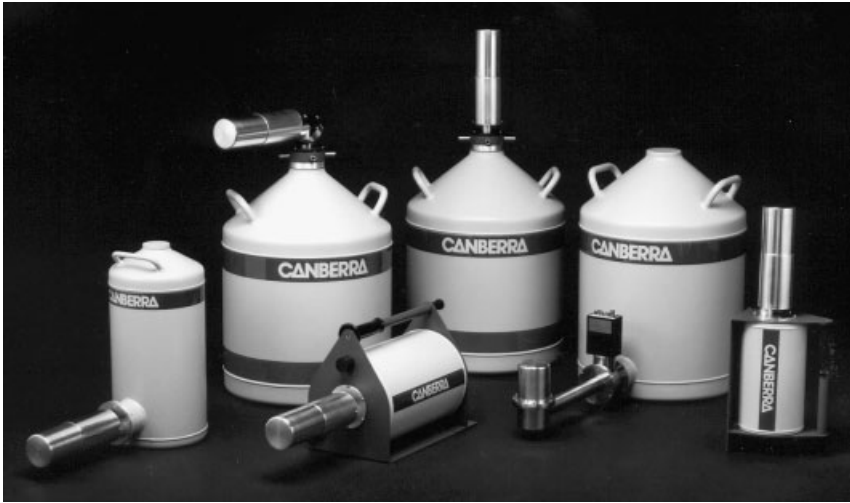
Fig. 10.23 Examples of HPGe detectors. (Courtesy Canberra, Inc.)
